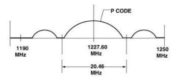
Figure 9-3. L2 Carrier Frequency.
