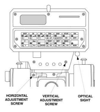
Figure 5-25. Adjusting Parallelism.
