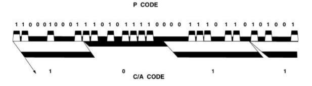
Figure 9-4. P Code and C/A Code Data Sequence.
