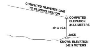
Figure 6-40. Elevation Error.
