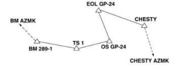
Figure 6-3. Closed Traverse on a Second Known Point.
