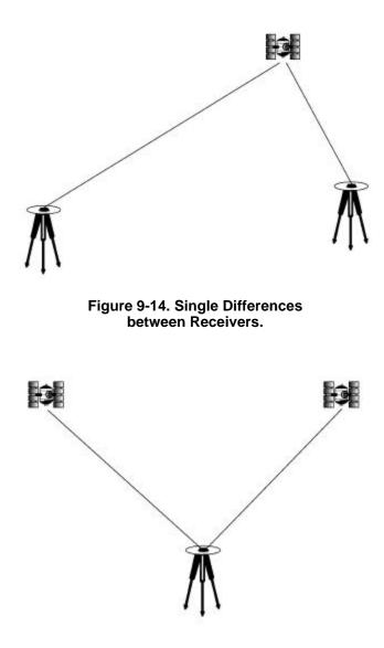
Figure 9-15. Single Differences between Satellites.
