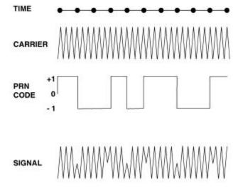
Figure 9-9. Carrier Modulated by PRN.
