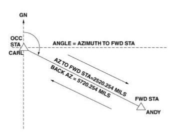
Figure 6-28. Azimuth.
