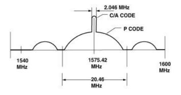
Figure 9-2. L1 Carrier Frequency.
