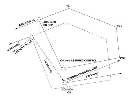
Figure 1-8. Swinging and Sliding the Grid.
