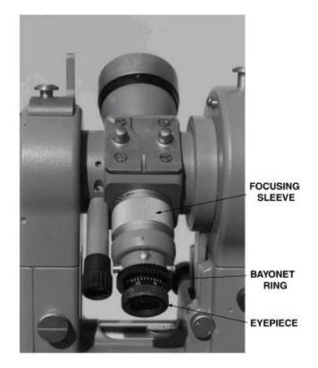
Figure 5-4. T-2E Focusing Sleeve and Eyepiece.
