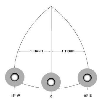
Figure 7-20. Time and Apparent Motion of the Sun.
