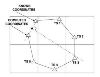
Figure 6-47. Determining the Error Station.
