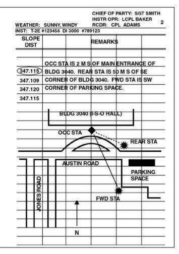
Figure 6-20. Example of an Angle Closed on the Horizon.
