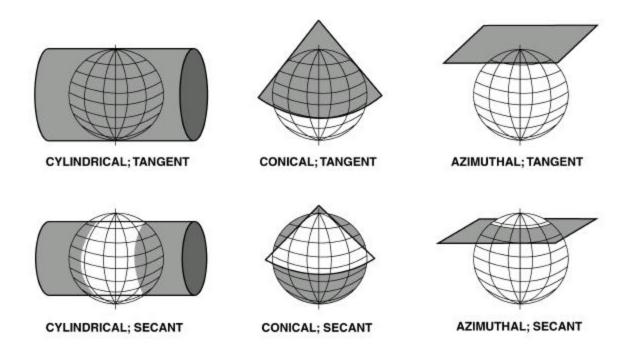
Figure 4-1. Projection Types: Tangent and Secant.
