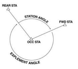
Figure 6-19. Angle Closed on the Horizon.
