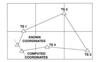
Figure 6-45. Determining the Error Leg -Parallel Line Method.
