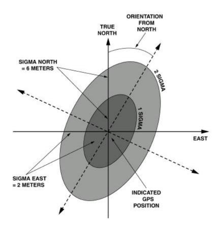
Figure 9-7. Error Ellipse at 2- $\sigma$  RMS.
