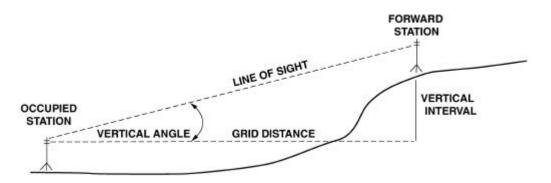
Figure 6-31. Elevation Triangle.
