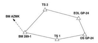
Figure 6-4. Closed Traverse on the Starting Point.
