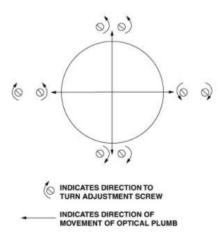
Figure 5-15. Optical Plumb Adjustment Screws.
