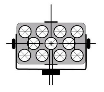
Figure 5-11. Pointings on an Eleven-Prism Holder (GPH11).
