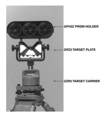
Figure 5-27. Target Set with GRZ3 and GPH3Z.
