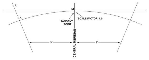
Figure 4-9. Line Distortion and Scale Factor in the GK Projection.
