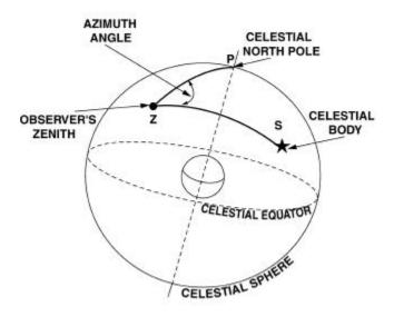
Figure 7-15. Azimuth Angle.
