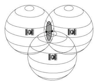
Figure 9-13. Ranging Three Satellites.
