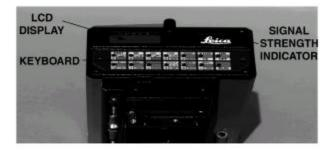
Figure 5-23. DI 3000 Control Panel.
