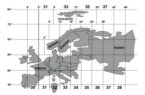
Figure 4-17. Nonstandard UTM Grid Zones.
