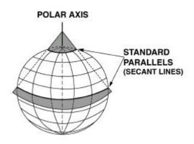
Figure 4-10. Secant Condition of Lambert Conformal Conic Projection.
