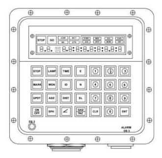
Figure 8-3. Control and Display Unit.
