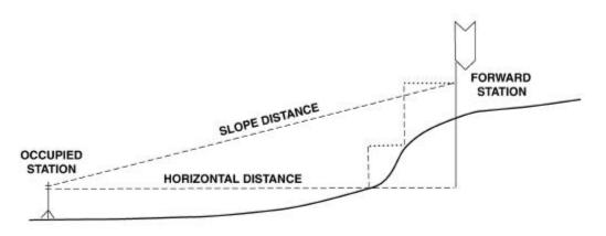
Figure 6-9. Slope and Horizontal Distances.
