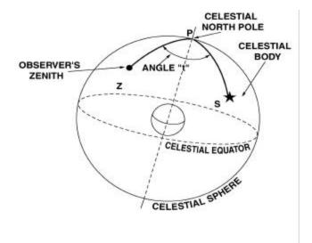
Figure 7-14. Hour Angle (Time Angle or Angle t).
