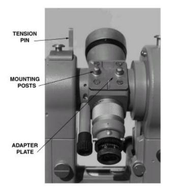
Figure 5-21. T-2E Modification for DI 3000.
