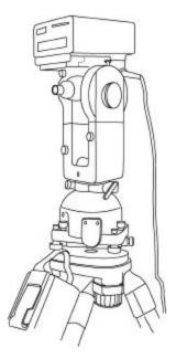
Figure 5-22. DI 3000 Mounted on T-2E.
