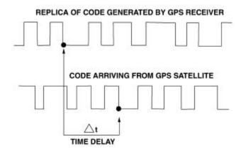
Figure 9-10. Time Delay of a GPS Signal.
