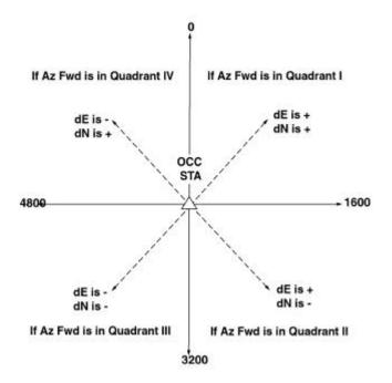
Figure 6-34. Determining the Sign of dE and dN.
