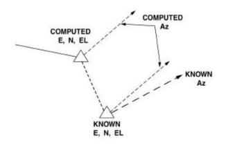
Figure 6-37. Traverse Closing Data Comparison.
