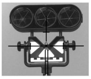
Figure 5-10. Pointings on a Target Reflector (GRZ3).
