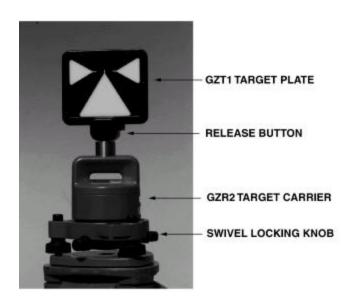
Figure 5-26. Target Set with Target Plate.
