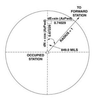
Figure 6-32. Value of Trigonometric Functions of Angles.
