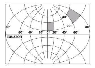
Figure 4-5. Distortion within the TM Projection.
