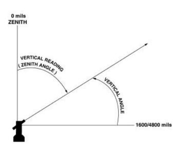
Figure 5-14. Vertical Readings/Angles.
